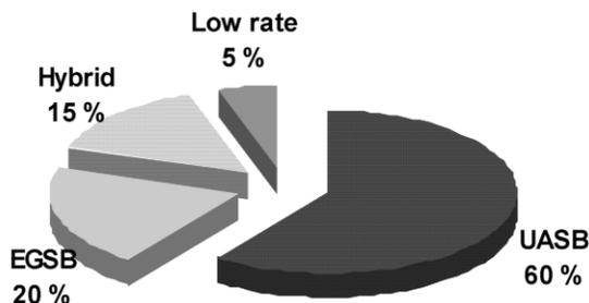
**Fig. 1** Distribution of modern anaerobic WWTPs (total: 20) constructed in Russia during 1998–2007 with regard to reactor type (updated from [6]).
