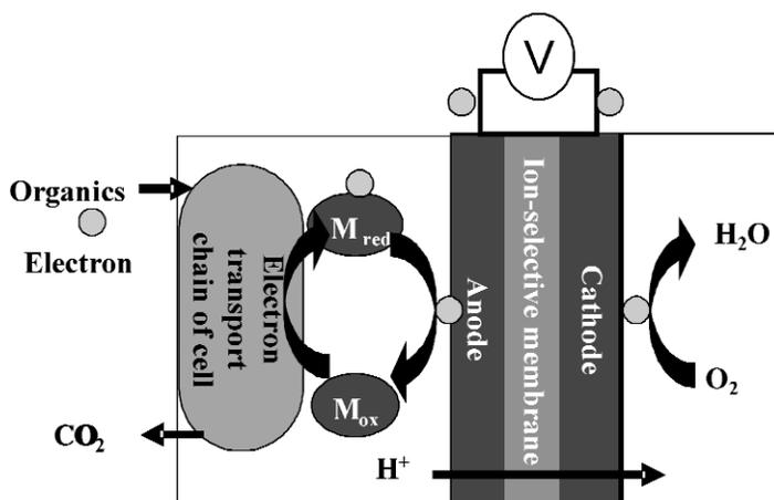
Fig. 3 Schematic representation of MFC.
