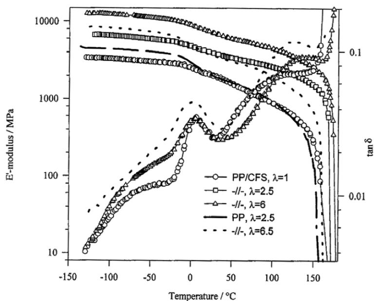
**Fig. 4** DMTA spectra of neat PP and PP + 20 wt % CFS composites. The initial isotropic specimen PP/CFS ( $\lambda = 1$ ) is compared with drawn ones of various draw ratios  $\lambda$  provided in the insert.  $E'$  in draw direction.
