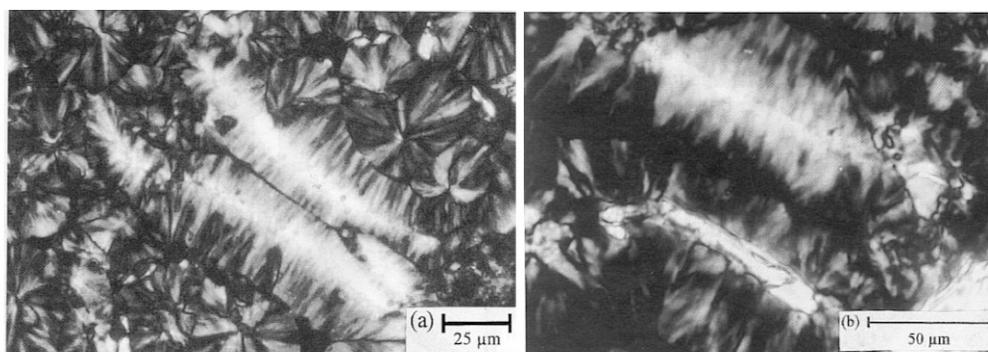
**Fig. 3** Optical micrographs showing the *trans*-crystallization in selected samples of (a) PP + 30 wt % XL and (b) PP + 30 wt % CFM composites.
