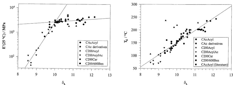
**Fig. 8** Storage modulus  $E'$  at 25 °C (left) and  $T_g$  (right) of a large number of mixed CA derivatives and acylates, carbanilates, benzoates, as a function of the interaction parameter  $\delta_L$ .
