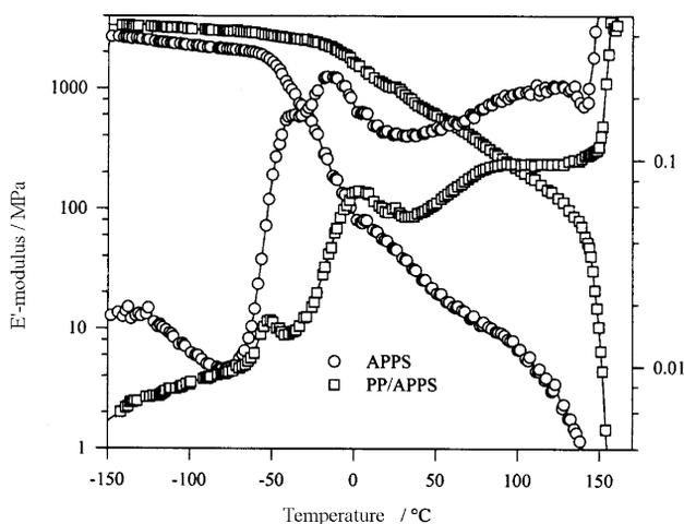
**Fig. 5** DMTA spectra of a so-called APPS and a mixture of PP and APPS (PP/40 wt % APPS).
