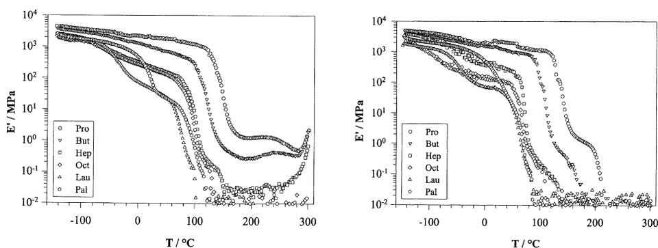
**Fig. 7** DMTA spectra of highly substituted cellulose propionate, butyrate, heptanoate, octanoate, laurate, and palmitate (DS = 2.8, left) and the fully substituted specimens with the remaining OH groups of the samples of the left picture acetylated (right).
