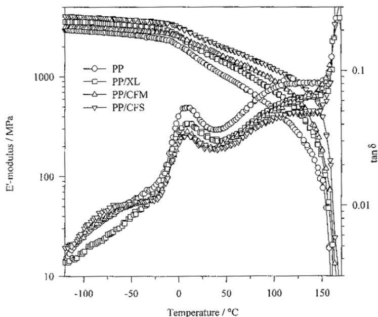
**Fig. 2** DMTA spectra with storage modulus  $E'$  (upper curves) and damping factor  $\tan\delta$  (lower curves) as a function of temperature for neat PP and PP + 30 wt % filler content (XL: xylan filler, CFM: microcrystalline cellulose, CFS: high-tenacity rayon fiber).
