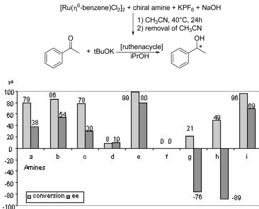
Fig. 4 HTE screening of chiral amines in Ru-catalyzed asymmetric transfer hydrogenation of acetophenone. Positive ee's correspond to the *R* configuration of 1-phenylethanol.
