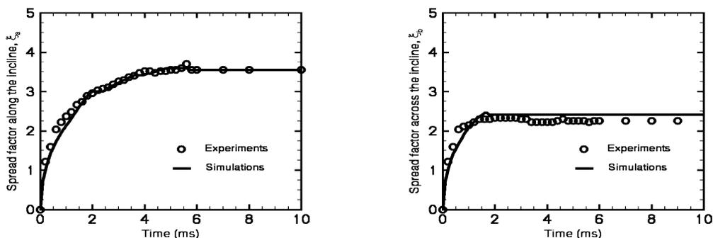
**Fig. 2** Comparison of the predicted and measured values of spread factor for tin drop impact of Fig. 2 (left: along the incline; right: across the incline).
