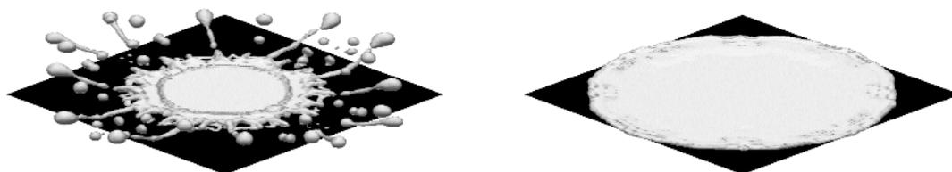
**Fig. 3** Predicted nickel splat shapes at two different substrate temperatures. Left: 290 °C; right: 400 °C.
