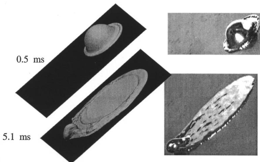
**Fig. 1** Comparison of the predicted (left column) and photographs (right column) of the impact of tin droplet on stainless steel substrate. Droplet diameter 2.2 mm; impact speed 2.35 m/s; initial drop temperature 240 °C; initial substrate temperature 25 °C; incline angle 45°.
