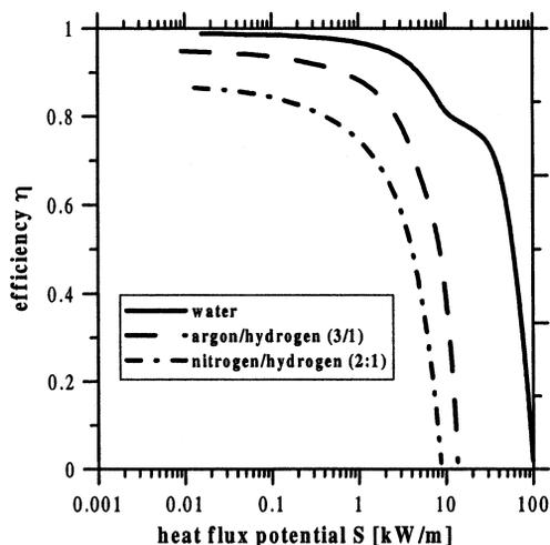
**Fig. 3** Dependence of thermal efficiency of plasma jet on heat flux potential for typical operation conditions of gas- and water-stabilized plasma spraying torches.
