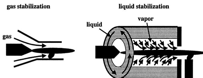
Fig. 1 Schematics of gas- and liquid-stabilized arcs.
