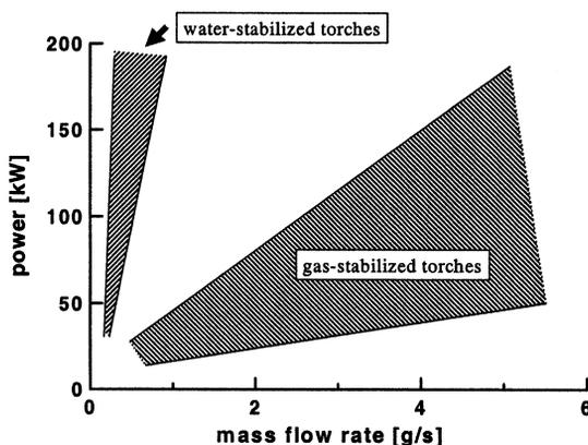
Fig. 2 Operation regimes of plasma spraying gas- and water-stabilized torches.
