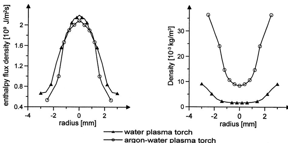
**Fig. 4** Radial profiles of enthalpy flux density and plasma density at the nozzle exit of water-stabilized and hybrid torch at arc current 400 A.
