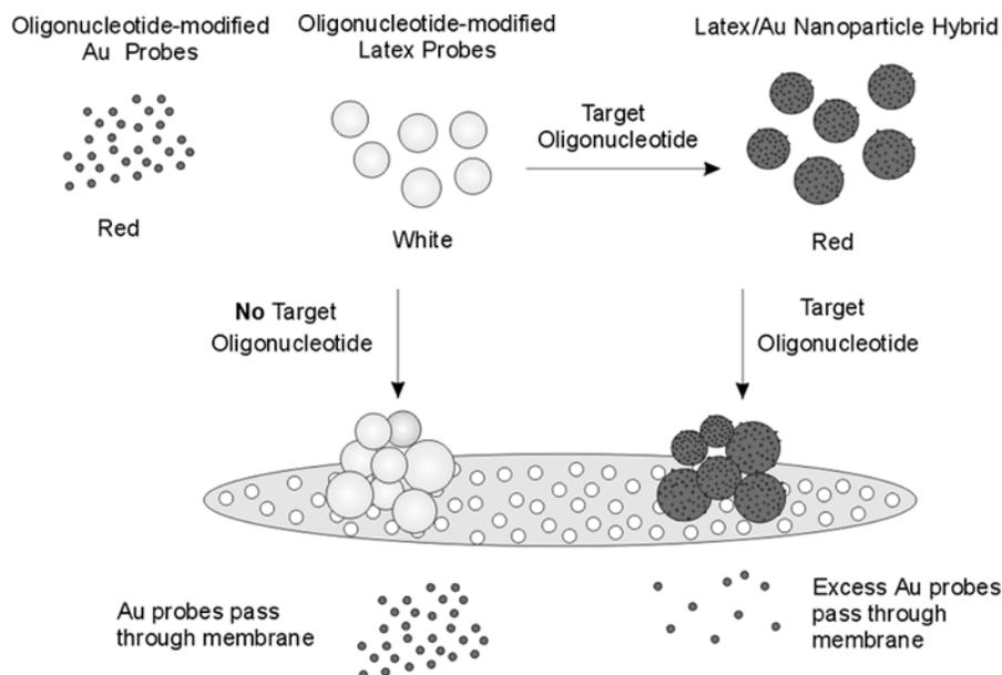
**Fig. 2** Gold nanoparticle/latex microsphere-based colorimetric DNA detection method.
