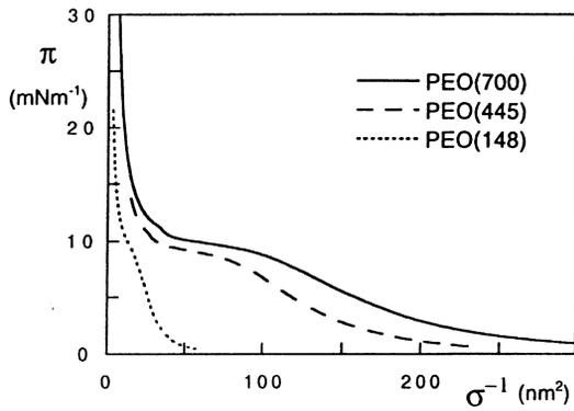
**Fig. 7** Surface pressure isotherms of the PS-PEO block copolymers.
