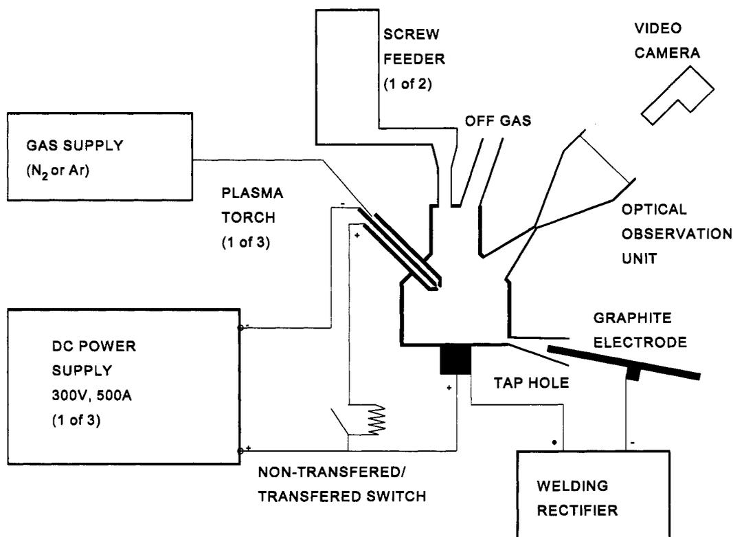
Fig. 1 PRESS plasma reactor facility at SINTEF
