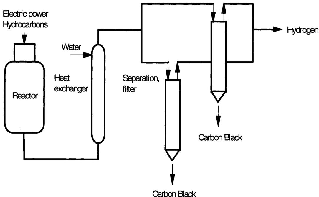
Fig. 6 Flow sheet for Kvaerner's plasma process for Carbon Black and hydrogen.
