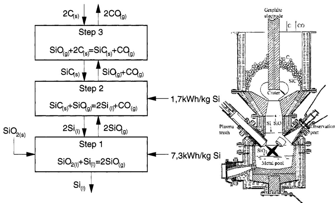
Fig. 3 Three-step plasma process for silicon metal production.
