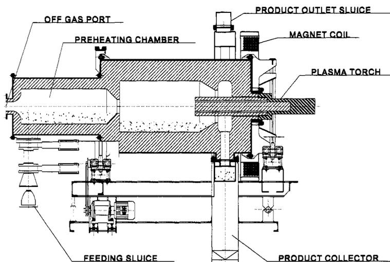
Fig. 8 Plasma rotary furnace.
