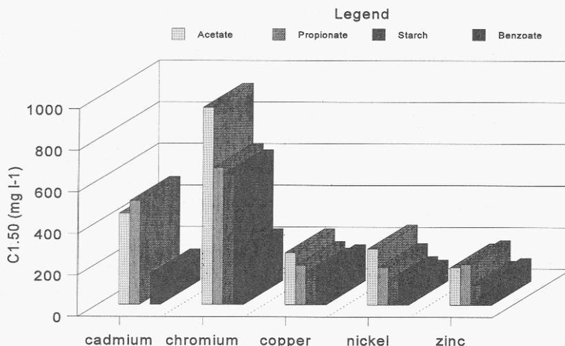
Fig.3.  $C_{1.50}$  values of heavy metals for various biogranules
