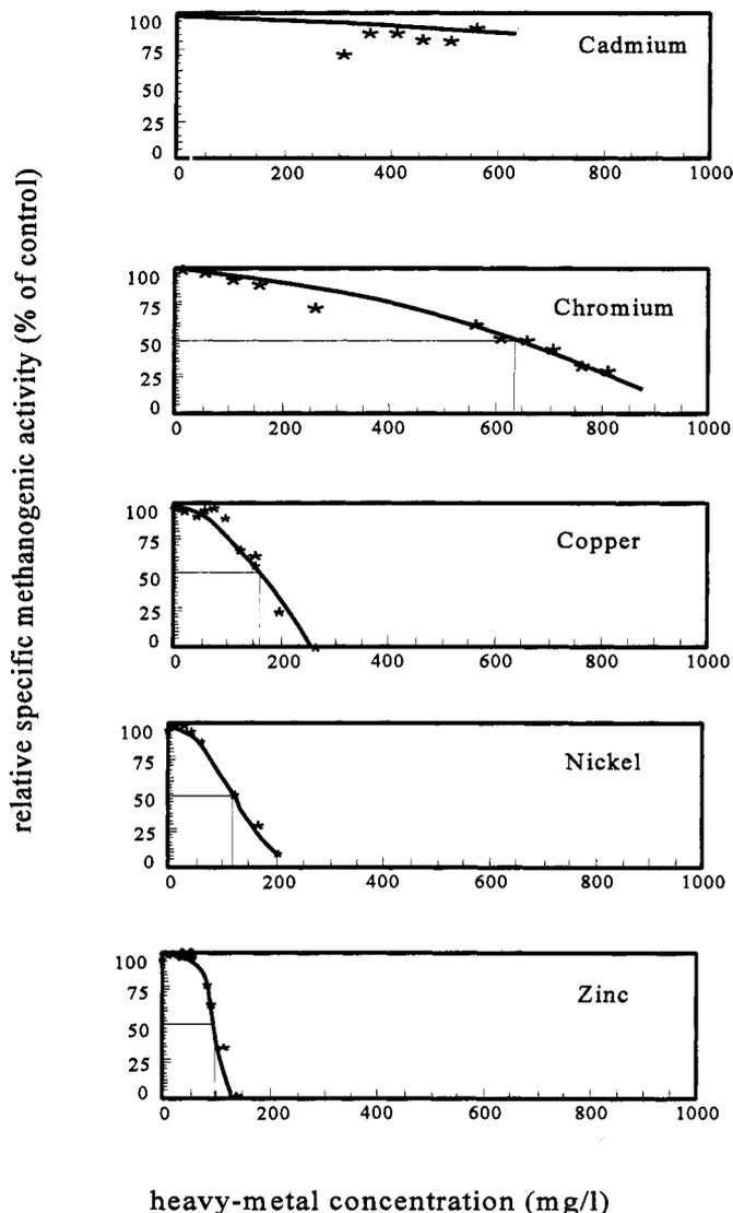
Fig.2. Reduction of specific methanogenic activity with increased metal concentration
