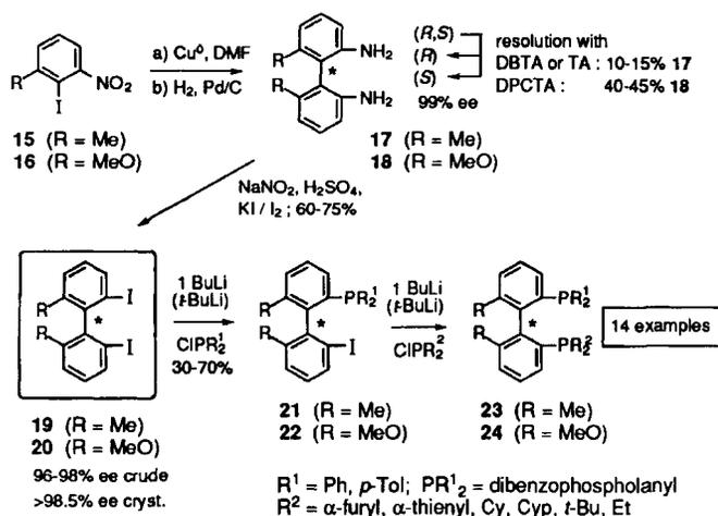
Fig. 5. Diiodide route to unsymmetrical biphenyl diphosphines
