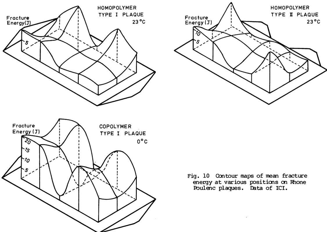
Fig. 10 Contour maps of mean fracture energy at various positions on Rhone Poulenc plaques. Data of ICI.
