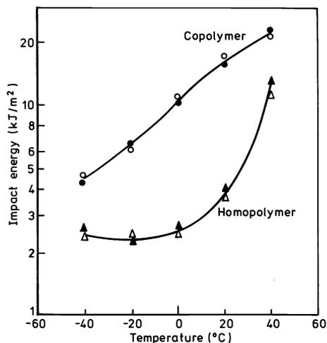
Fig. 8 Charpy impact energy of compression moulded polypropylene bars with 2mm radius notch. Ageing time: (o, Δ) 1 week; (●, ▲) 10 weeks. Data of TNO.
