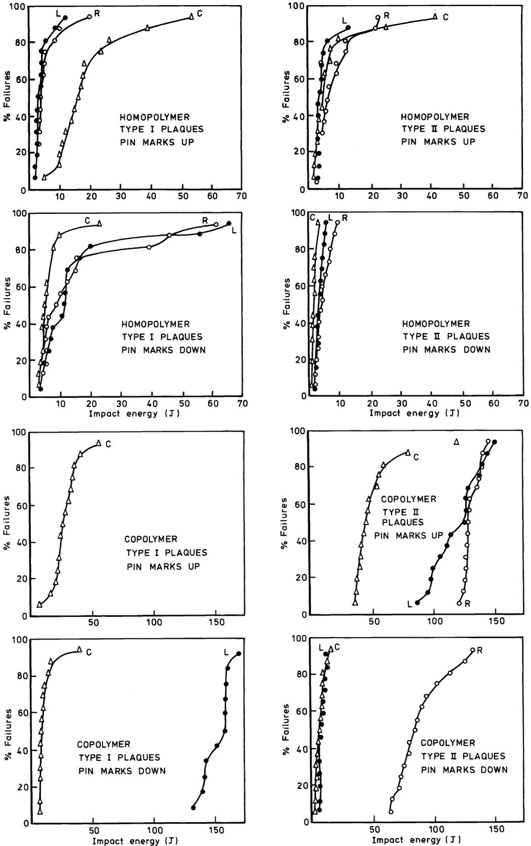
Fig. 12 Driven dart impact data for specimens from Rhone-Poulenc plaques. Note difference in energy scale between homopolymer and copolymer. Specimens are struck on upper face. L, C and R as defined in Fig. 11. Data of Monsanto.
