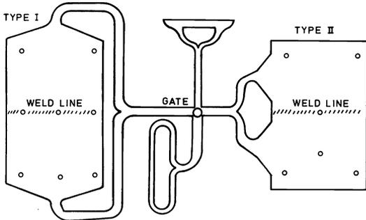
Fig. 1 The Rhone-Poulenc double-gated plaque mould, showing ejector pin positions.
