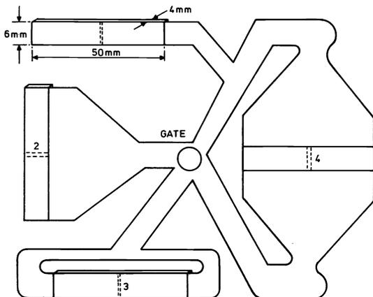
Fig. 2 The ICI multi-cavity mould, showing the labelling of positions. Bars are identical in size. Double lines show locations of moulded in notches on upper face.
