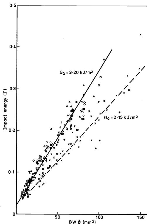
Fig. 7 Charpy impact data for copolymer, obtained by Hoechst. Ageing time (days): (o) 1; (●) 2; (□) 4; (■) 8; (◇) 16; (∇) 130; (Δ) 135; (X,+), 700.
