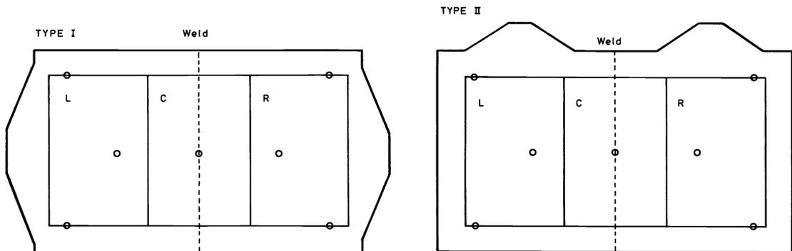
Fig. 11 Cutting plan for Monsanto driven dart specimens.
