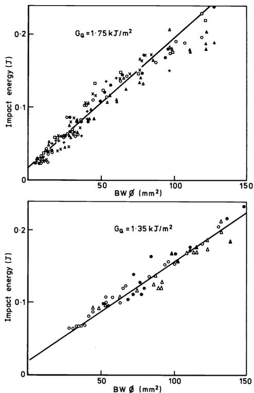
Fig. 6 Charpy impact data for homopolymer, obtained by Hoechst. Top: short-term ageing (in days) (X) 1; (o) 2; (+) 4; (●) 8; (□) 16; (▲) 130; (Δ) 135. Bottom: aged for 2 years, with B X W(mm) = (o) 6 X 4; (●) 10 X 4; (Δ) 6 X 6; (▲) 10 X 6.
