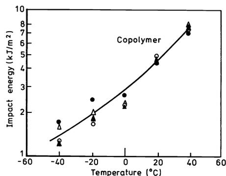
Fig. 9 Charpy impact energy of copolymer specimens with moulded-in notch from ICI multicavity mould. Data of TNO. Positions as shown in Fig. 2: (o) 1; (Δ) 2; (●) 3; (▲) 4.
