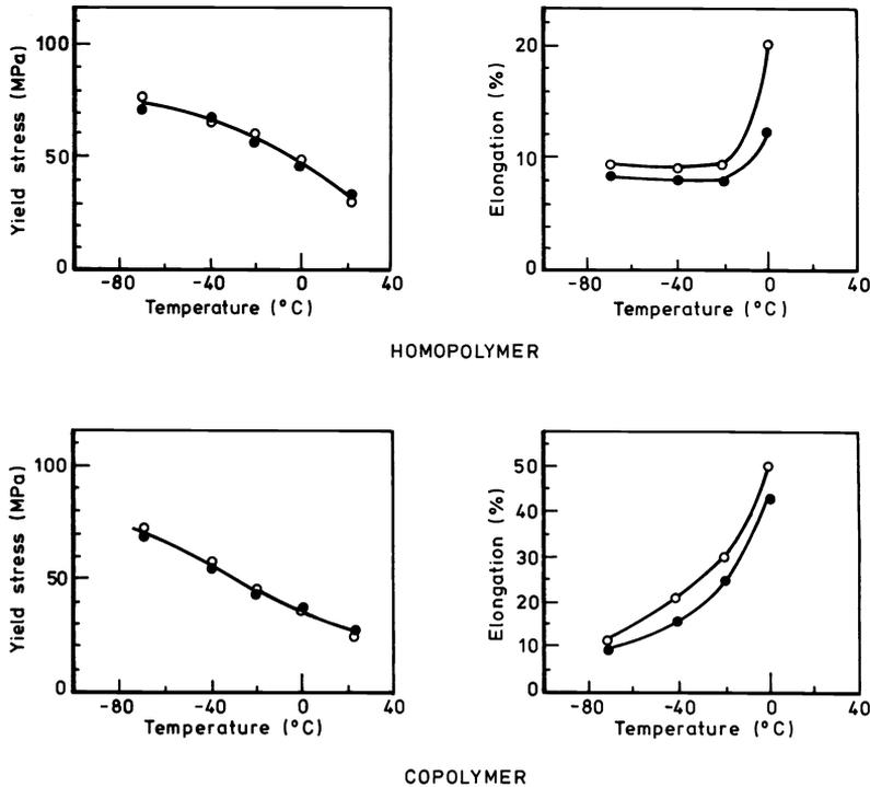
Fig. 5 Yield stress and elongation at break at low strain rate: along (○) and across (●) flow direction. Data of MP.
