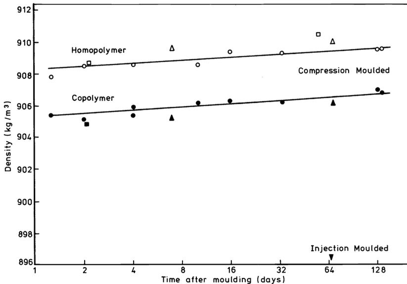
Fig. 4 Changes in density with time after moulding. Data of: (□, ■) BP; (○, ●) Hoechst; (△, ▲, ▼) TNO.
