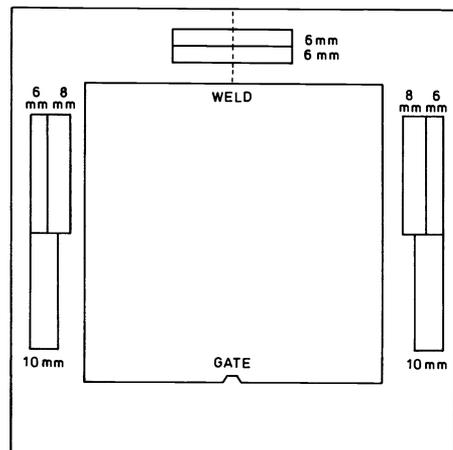
Fig. 3 The ICI picture frame mould, showing positions from which Charpy bars were cut by BP.
