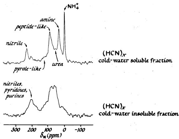
Fig.3 9.12-MHz  $^{15}\text{N}$ -NMR spectra of two fractions of the solid product of the reaction of hydrogen cyanide and anhydrous ammonia. Several hundred thousand 3-ms single matched cross-polarization contacts (with 30-kHz  $\text{H}_1$ 's) were used for each spectrum. The 300-mg samples were spun at 1.4 kHz.
