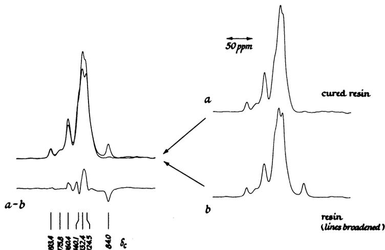
Fig.1. Cured Thermid 600 resin (a) and the resin before curing (b). The resin spectrum has been artificially broadened to facilitate comparison. The two spectra are also shown superimposed and their difference (a-b) is plotted. The net area of the difference spectrum is zero.
