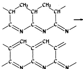
The effect of oxidation on Orlon 42, primarily polyacrylonitrile, is shown by the  $^{13}\text{C}$ -NMR spectra in Fig.2 (Ref.7). The Orlon 42 spectrum reveals an aliphatic region (up-field, to
