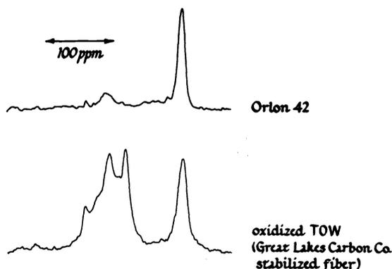
Fig. 2. 15.1-MHz  $^{13}\text{C}$ -NMR spectra of Orlon 42 before and after low temperature pyrolysis in air. Approximately 50 000 2-ms single matched cross-polarization contacts (with 40-kHz  $\text{H}_1$ 's) were used for each spectrum. Spinning was at 2 kHz.
