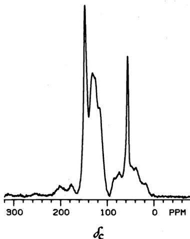
Fig.4. 15.1-MHz  $^{13}\text{C}$ -NMR spectrum of lignin. The sample was spun at 833Hz. The resulting spinning side bands were isolated by suitable PASS sequences and the side-band intensities returned to the center bands.
