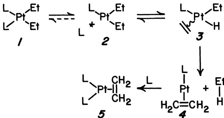
Fig. 2. Mechanism of thermal decomposition of  $\text{L}_2\text{PtEt}_2$  in cyclohexane solution ( $T = 141^\circ\text{C}$ ). Analogous mechanisms apply to other  $\beta$ -hydride elimination reactions.
