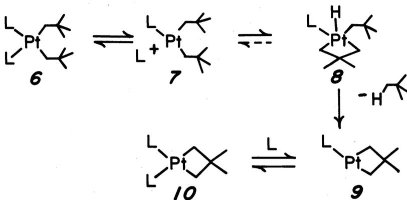
Fig. 4. Mechanism of thermal decomposition of dineopentylbis(triethylphosphine)platinum(II).
