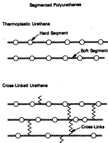
Fig. 4. Generalized form of thermoplastic and cross-linked urethanes.
