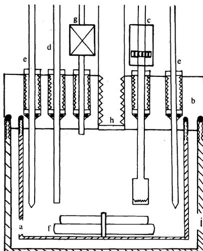
Fig. 7. Schematic diagram of a gas solution calorimeter (Cone et al. (11)).
