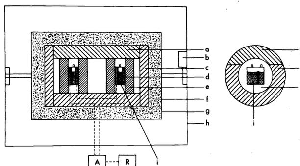
Fig. 2. Batch heat conduction calorimeter for mixing of two liquids (Ref. 6; LKB 2107). (left) longitudinal section. (a) aluminium cover, (b) rotation motor, (c) aluminium heat sink, (d) semiconductor thermopiles, (e) aluminium block, (f) styrofoam insulation, (g) stainless steel container, (h) thermostated air or water bath, (i) reaction vessel. A is an amplifier och R is a recorder/integrator. (right) transverse section through calorimeter block.
