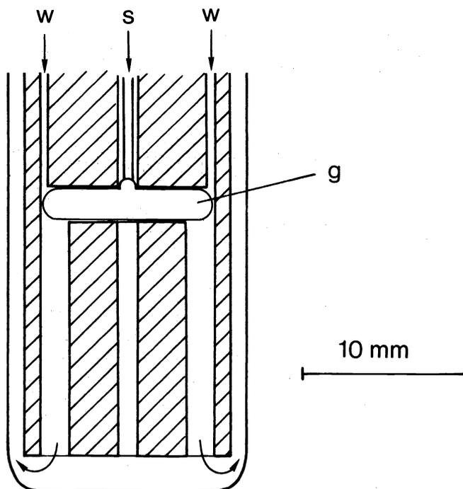
Fig. 8. Schematic view of the solution zone of a new flow solution calorimeter for slightly soluble gases (18).
