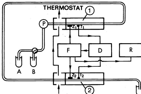
Fig. 9. Principle of the Picker flow heat capacity calorimeter. (A) solvent, (B) solution, ( $Z_1, Z_2$ ) heaters, ( $T_1, T_2$ ) thermistors, (P) pump, (F) feed back, (D) null detector, (R) recorder.
