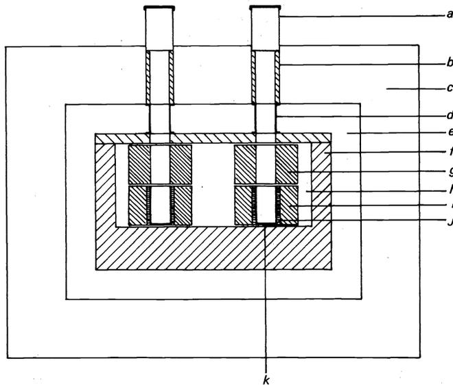
Fig. 5. Twin heat conduction calorimeter used for insertion of ampoules or flow vessels (12). (a) steel tube, (b) copper constriction, (c) water thermostat, (d) steel tube, (e) air space, (f) main heat sink, (g) aluminium block, (h) air space, (i) air space, (j) thermocouple plate, (k) ampoule holder.
