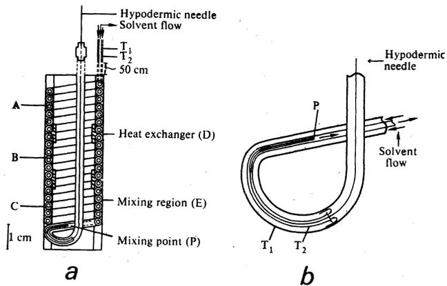
Fig. 4. Flow vessel for solution of slightly soluble liquids. (a) Section through the vessel. (b) Details of the mixing region. Reprinted from (11).
