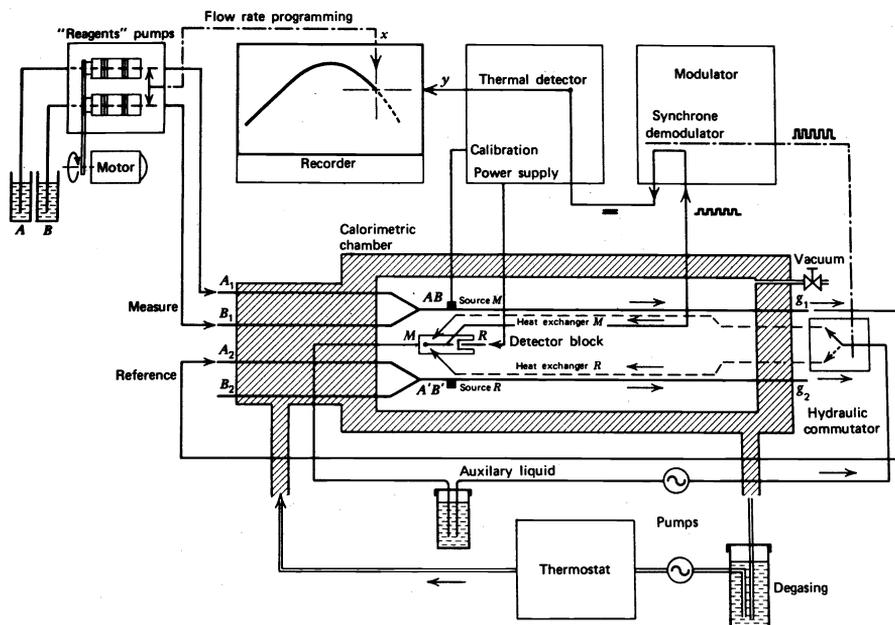
Fig. 3. Principle of the Picker flow mixing calorimeter (9,10).
