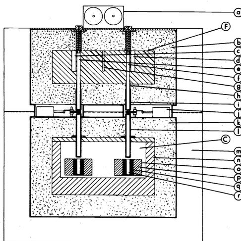
Fig. 10. Schematic view of a twin drop heat capacity calorimeter for small samples (23).
