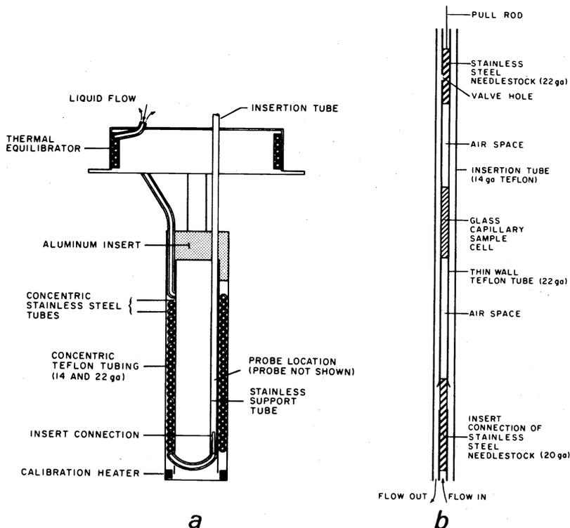
Fig. 6. Flow vessel for solution of small samples of slightly soluble solids (Gill and Seibold). (a) Section through the vessel. (b) Expanded view of the solid insert probe. Reprinted from (15).
