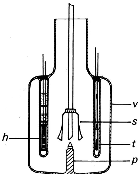
Fig. 1. A typical reaction vessel for a conventional solution calorimeter (LKB 8721-1).
