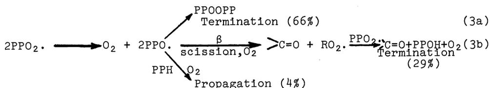
radical ( $\text{RO}_2$ , reaction 3b). The percentages are taken from ref. (3) and are for atactic PPH at  $45^\circ\text{C}$  with a thermal initiator.
