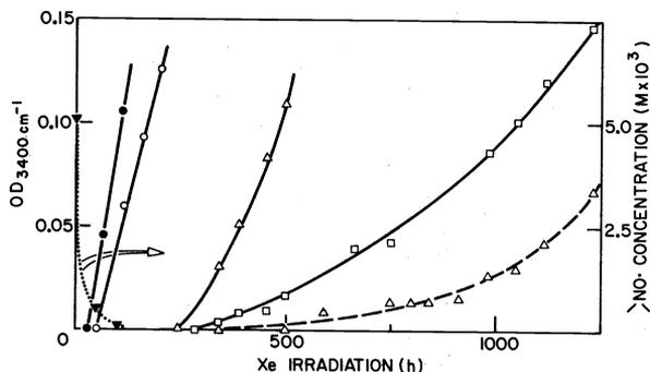
Fig. 4. Stabilization of PPH by piperidine species. Film samples (25  $\mu\text{m}$ ) irradiated in a xenon arc Weather-Ometer. Oxidation measured by  $-\text{OH}+\text{OOH}$  accumulation in the infrared at  $3400\text{ cm}^{-1}$ .
