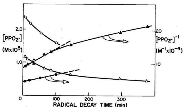
Fig. 3.  $\text{PPO}_2$  decay at  $25^\circ\text{C}$  by e.s.r. spectroscopy.  $\Delta\Delta$  Isotactic PPH film. Decay immediately after irradiation in a xenon arc Weather-Ometer for  $\sim 60$ h to  $0.12\text{M}$  in  $-\text{OOH}$  groups.  $\bullet\bullet$  Atactic PPH powder. Decay immediately after  $\gamma$ -irradiation in air (30 min at  $8000 \text{ rad. min}^{-1}$ ).
