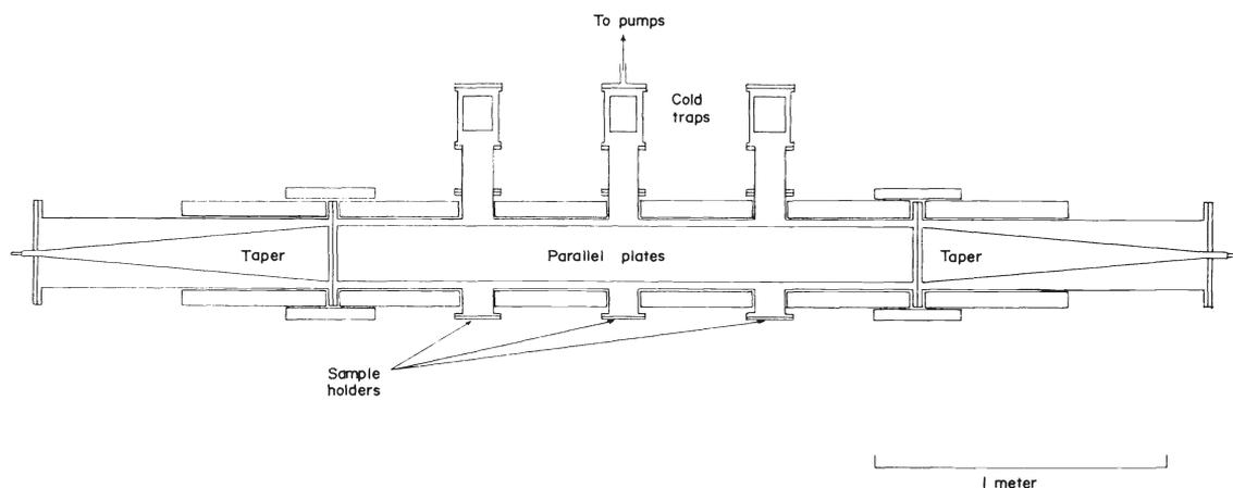
Fig. 7 (a). Heated parallel-plate cell used for studying the microwave spectrum of glycine.
