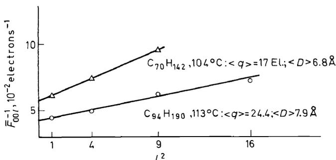
*Figure 12.* Plot for evaluating the average scattering power  $\langle q \rangle$  and the average depth  $\langle D \rangle$  of the 'holes' between the paraffin lamellae<sup>29</sup>.
