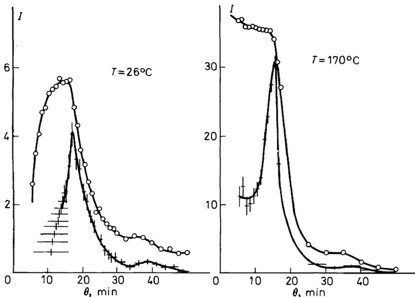
Figure 4. Examples of changes in SAXS curves by use of slit-correction:  $\circ$ - $\circ$ - $\circ$  measured intensity  $\text{---}+\text{---}+$  corrected pinhole scattering curve, the bars indicate the statistical confidence regions of the calculated data. Scattering curves were obtained from melt crystallized polyoxymethylene measured at the indicated temperatures<sup>57</sup>.
