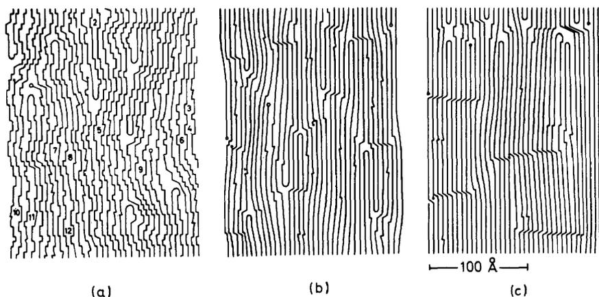
Figure 2. Suggested models of various states of polyethylene: (a) in the melt, (b) in the solid state at temperatures near the melting point, (c) in the solid state at low temperatures (after W. Pechhold and S. Blasenbrey<sup>2</sup>).
