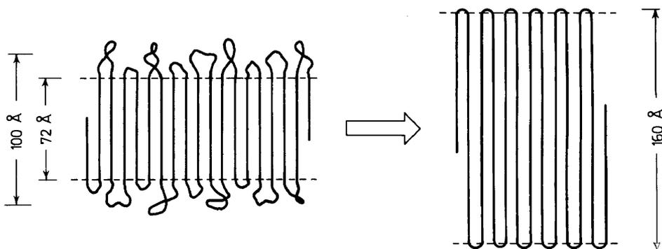
Figure 9. Schematic diagram showing the tightening of loose loops during the solid state transformation of the crystal modification of *trans*-1,4-polybutadiene (after Takayanagi *et al.*<sup>21</sup>).
