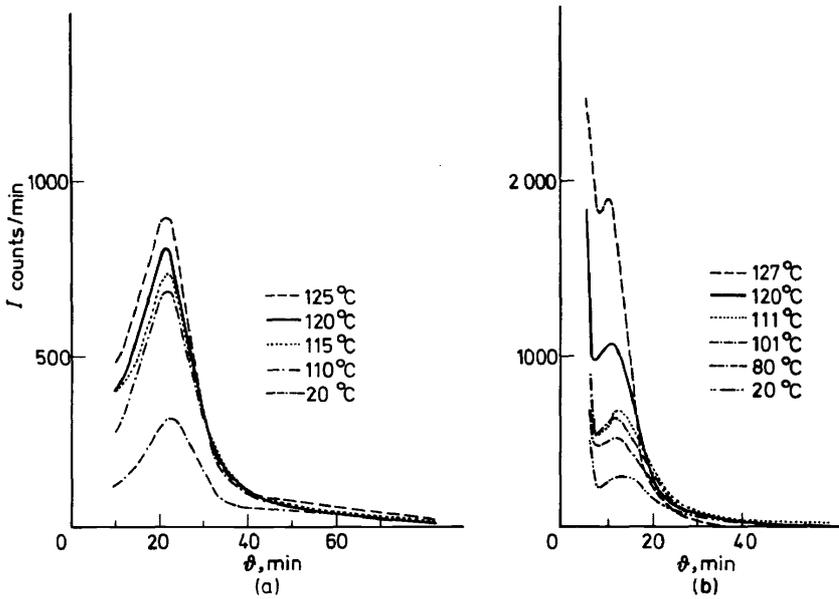
Figure 26. SAXS curves of polyethylene single crystals measured at various temperatures<sup>56</sup>. The samples were annealed before measuring at (a) 125°C, (b) 130°C.
