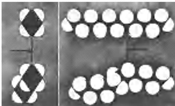
Figure 16. Model of a kink defect. Left hand: planar paraffin chain; right hand: paraffin chain with a  $2g1$ -kink isomer (after W. Pechhold *et al.*<sup>2</sup>).
