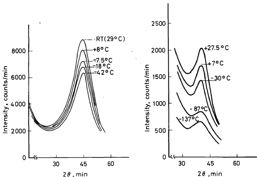
Figure 6. SAXS curves of solution grown polyethylene crystals measured at various temperatures<sup>15</sup>: (a) branched, (b) linear polyethylene.
