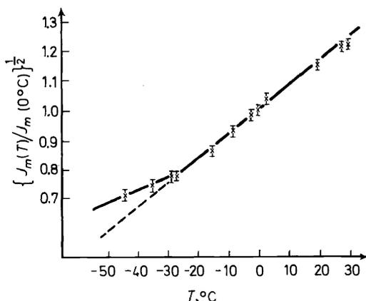
*Figure 5.* Relative change in peak intensity of the long spacing reflection of polybutene-1 single crystals as a function of temperature<sup>13</sup>.
