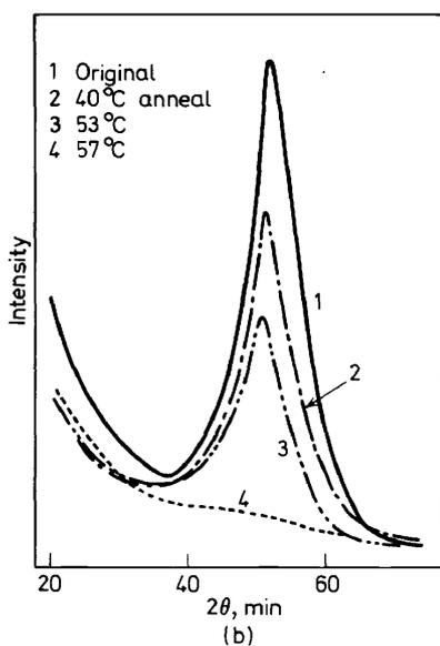
Figure 8. Annealing behaviour of single crystals of *trans*-1,4-polybutadiene (after Takayanagi *et al.*<sup>21</sup>). (a)  $\tan \delta$  curves of single crystals annealed at various temperatures; (b) SAXS curves of single crystals annealed at various temperatures.
