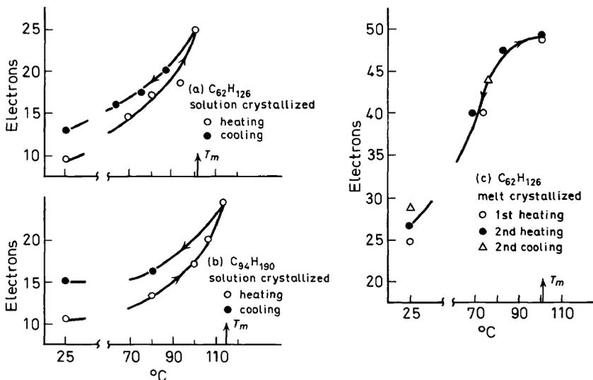
Figure 20. Dependence of the average scattering power  $\langle q \rangle$  of *n*-paraffin samples on temperature during heating and cooling cycles (after measurements by G. R. Strobl<sup>29</sup>).
