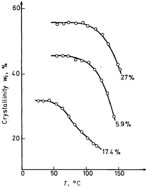
Figure 25. Variation of the degree of crystallinity of trioxan-dioxolane copolymers with temperature<sup>44</sup>.
