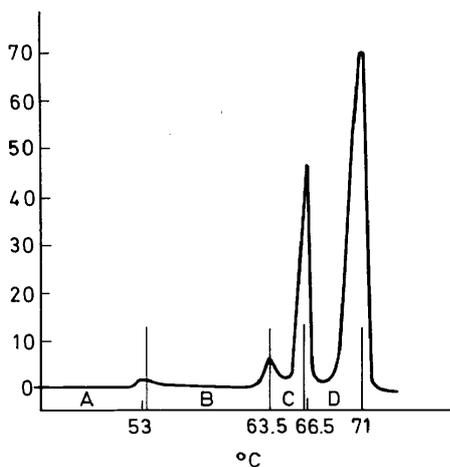
Figure 13. Differential scanning calorimeter curve of a melt crystallized  $n$ -tritriacontane  $C_{33}H_{68}$  showing the existence of four crystalline modifications A, B, C and D (after G. R. Strobl<sup>29</sup>).
