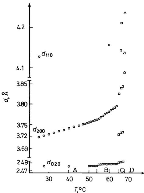
Figure 14. The spacings of (110), (200) and (020) net planes of  $C_{33}H_{68}$  as a function of temperature<sup>30</sup> showing the splitting of the reflection at the transitions B  $\rightarrow$  C and C  $\rightarrow$  D.  $\circ$  Modification A and B,  $\square$  Modification C,  $\triangle$  Modification D ('rotational' phase).
