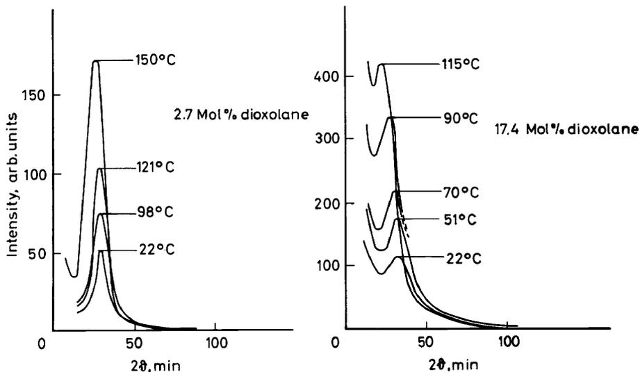
*Figure 27.* Slit-corrected SAXS curves of trioxan-dioxolane copolymers measured at the indicated temperatures<sup>44</sup>.
