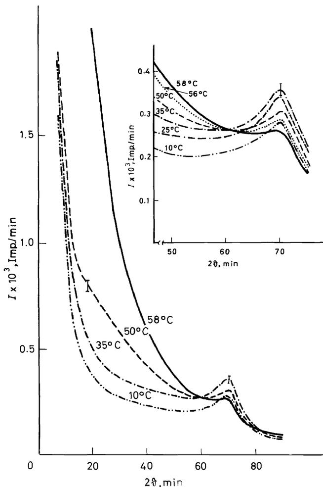
Figure 30. SAXS curves of polyethylene oxide single crystals measured at the indicated temperatures<sup>4,5</sup>.
