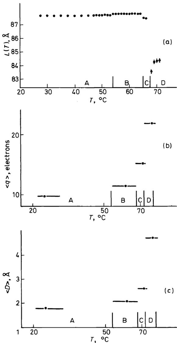
Figure 15. Temperature dependence of the small angle x-ray scattering of melt crystallized  $C_{33}H_{68}$ : (a) Long spacing  $L$ , (b) Average scattering power  $\langle q \rangle$  per chain, (c) Average depth of the scattering interlamellar region.
