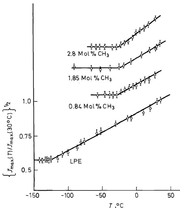
Figure 7. The temperature dependence of the peak intensity of the long spacing reflection of solution crystallized polyethylenes possessing the indicated degrees of CH<sub>3</sub>-branching (curves of branched PE are shifted for 0.2 unit along the ordinate).
