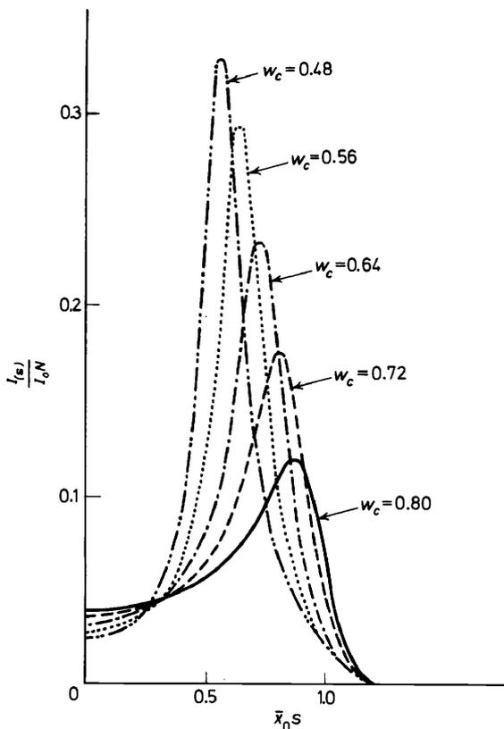
*Figure 32.* Dependence of calculated scattering curves on degree of crystallinity  $w_c$ . The curves were calculated assuming that the decrease in crystallinity is due to an increase in thickness of the amorphous intercrystalline layers<sup>54</sup>.
