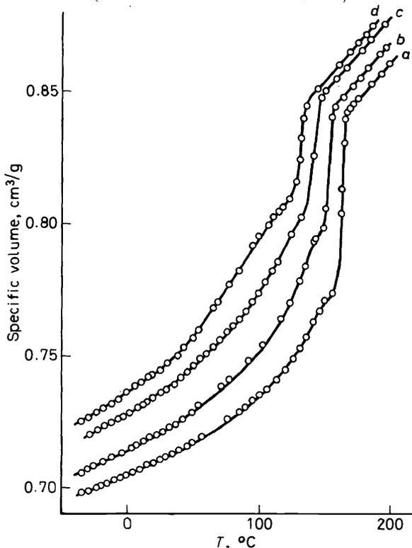
Figure 24. Specific volume of trioxan-dioxolane copolymers as a function of temperature (according to measurements by H. Wilski<sup>43</sup>): (a) 2.7 Mol% dioxolane, annealed at 150°C, (b) 5.9 Mol% dioxolane, annealed at 147°C, (c) 11.0 Mol% dioxolane, annealed at 134°C, (d) 17.4 Mol% dioxolane, annealed at 121°C.
