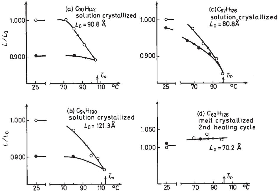
Figure 18. The relative changes in long spacings of *n*-paraffin crystals depending on temperature (according to measurements by G. R. Strobl<sup>29</sup>):  $\circ$  heating  $\bullet$  cooling.
