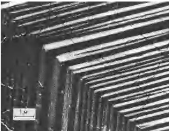
Figure 19. Surface replica of a  $\text{C}_{94}\text{H}_{190}$  crystal after heating to 110  $^{\circ}\text{C}$  (electron micrograph by I. G. Voigt-Martin<sup>30</sup>).
