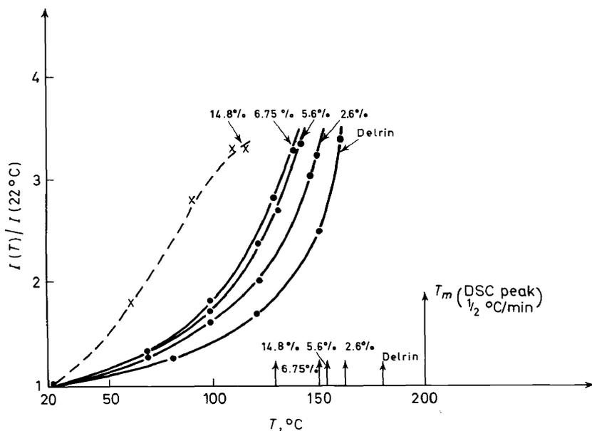
Figure 28. Variation of the relative peak intensity of the small angle reflection with temperature<sup>44</sup>. The arrows indicate the DSC-melting points of the various trioxan-dioxolane copolymers.
