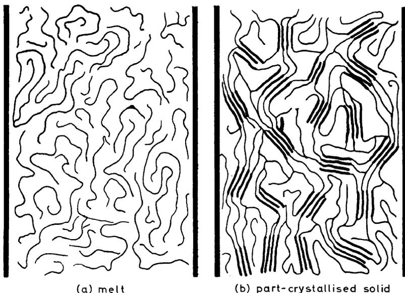
*Figure 1.* Model of the changes in structure during melting and crystallization of polymers (after A. R. Ubbelohde<sup>1</sup>).
