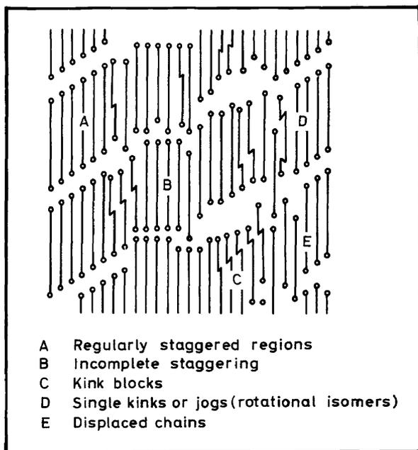
Figure 22. Schematic drawing of the structure of a long chain paraffin crystal at a temperature some degrees below the melting point.
