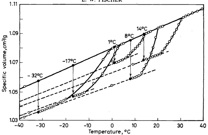
Figure 23. Melting curves of natural rubber as a function of crystallization temperature (after L. A. Wood and N. Bekkedahl<sup>42</sup>).
