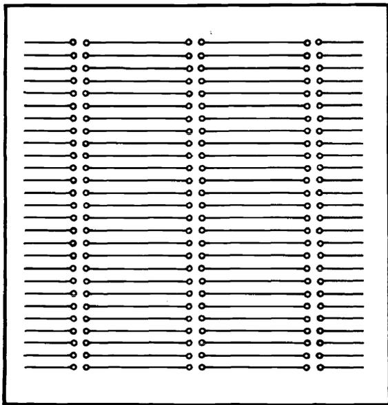
*Figure 21.* Schematic drawing of the structure of a long chain paraffin crystal at room temperature (orthorhombic modification).
