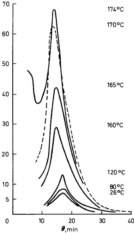
Figure 31. Slit corrected SAXS curves of polyoxymethylene (Delrin) measured at the indicated temperatures<sup>57</sup>.
