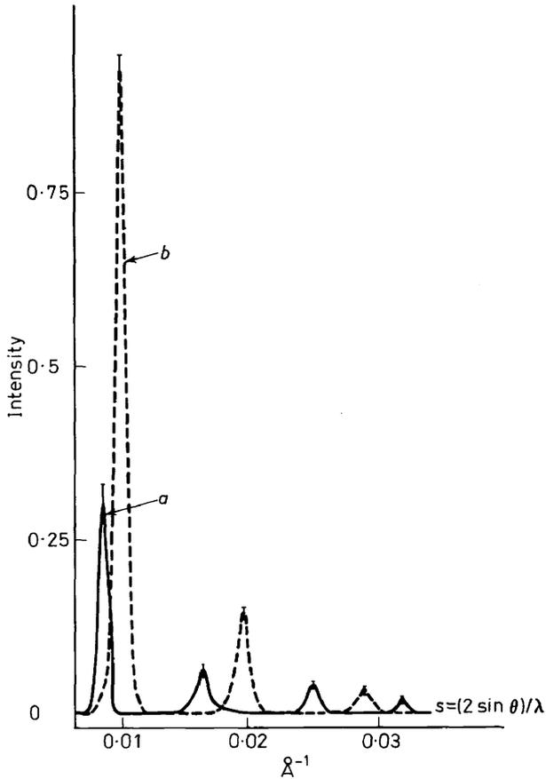
Figure 11. Slit-corrected SAXS curves of solution crystallized  $C_{94}H_{190}$  (background scattering subtracted): *a* measured at room temperature; *b* measured at  $110^{\circ}C$  (according to measurements of G. R. Strobl<sup>29</sup>).
