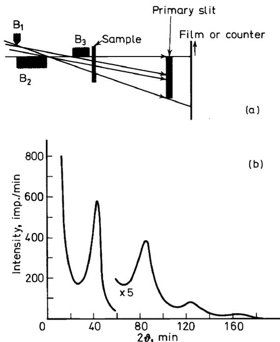
Figure 3. (a) Schematic drawing of a small angle x-ray scattering camera with slit collimation (after O. Kratky<sup>4</sup>). (b) SAXS curve of a mat of polyethylene single crystals grown from dilute solutions<sup>5</sup>.
