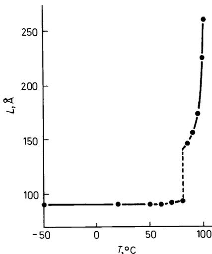
Figure 10. Long spacing of single crystals of isotactic polybutene-1 as a function of temperature<sup>24</sup>.
