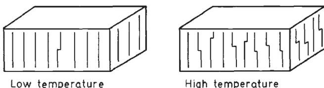
Figure 17. Schematic structure models of a paraffin lamella below and above the transition temperature<sup>35</sup> (the increased roughness of the surface is not taken into account in this drawing).
