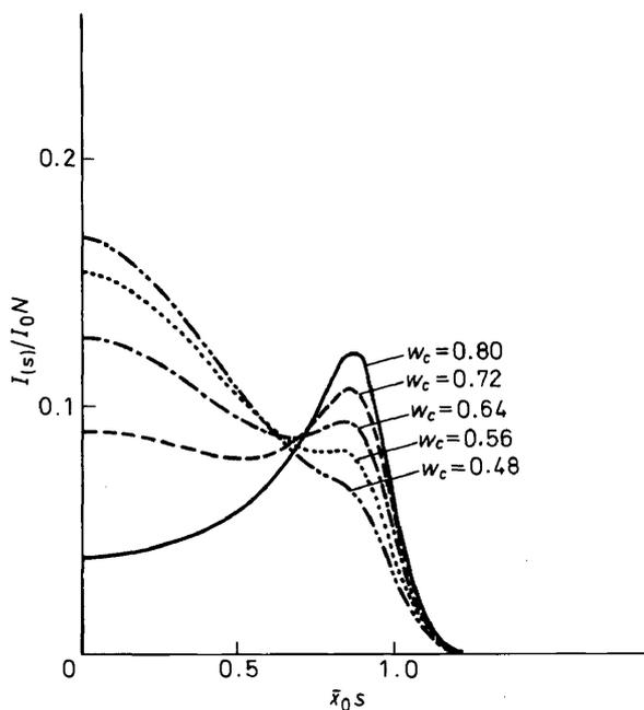
Figure 29. Dependence of calculated scattering curves on degree of crystallinity  $w_c$ . The curves were calculated using the assumption that some statistically distributed crystallites melt completely<sup>54</sup>.
